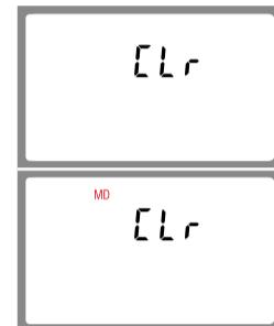
From the set-up menu, use **M** and **P** buttons to select the reset option.
