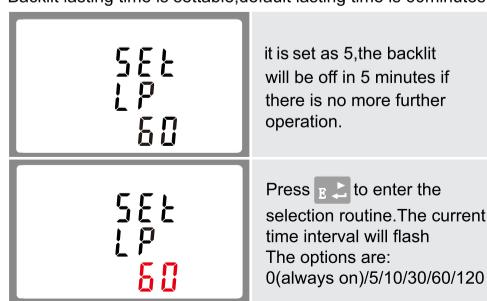
Press **M** and **P** to select the time interval. Then press **E** to confirm the set-up.
