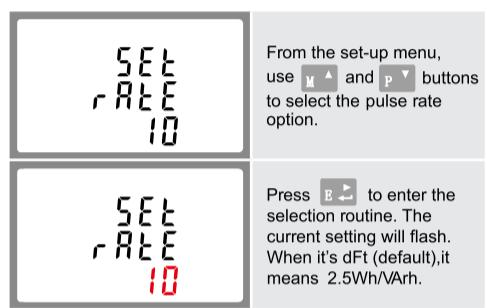
Use **M** and **P** buttons to choose pulse rate, then press **E** to confirm the setting and press **W1** to return to the main set up menu.
