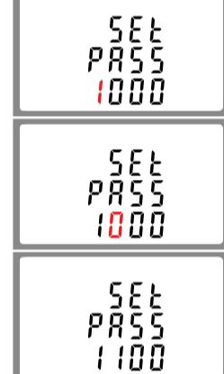
Press the **E** to enter the change password routine. The new password screen will appear with the first digit flashing.
